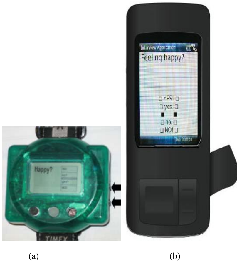
Figure 23. Two platforms that were explored during the EMA development process: (a) the eWatch and (b) a smartphone with a silicon sleeve button interface (right). Both platforms are displaying an example question of the interview application
